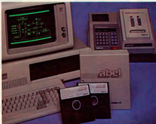
ABEL is also available as part of complete development system that allows the engineer to design, program and test more than 130 logic devices.
