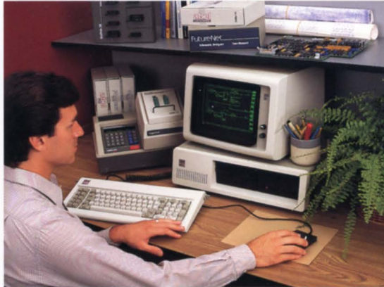
A complete Personal Silicon Foundry fits on your desk and contains all the hardware and software needed for design, programming and testing of PLDs.
