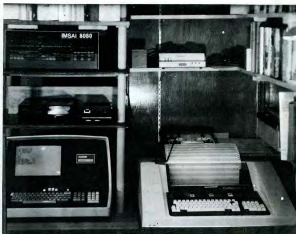
The Sherry Bros. #2 system. This features an Imsai Mainframe, A.D.D.S. terminal, Pennywhistle Modem, Carterfone 1030 hardcopy unit and audio cassette.
