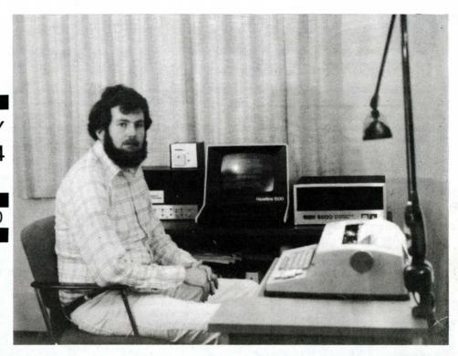
My system is a Southwest Tech 6800 with 36k of memory, dual mini floppys, a Hazeltine 1500 video terminal, and a Trendata 1000 Selectric terminal. The small box on the disk drive is my low cost modem
