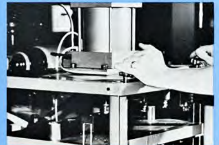
6. Insert template and PC board into air press for staking.
