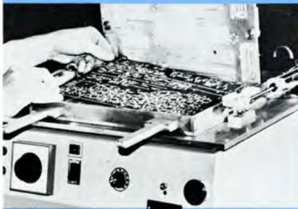
1. Place the PC board under the template of the Molex vibrator.
