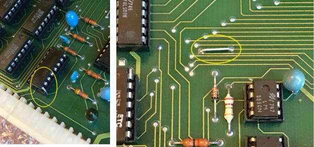
This mod connects the head load output (HLD) of the 1771 (pin 28) to U1 pin 1, replacing the FKTR00 signal previously connected to U1 pin 1. FKTR00 comes from U21 pin 9 which is disconnected by lifting the pin out of its socket. The HLD signal is picked up at a feedthru going to U9 pin 1.
