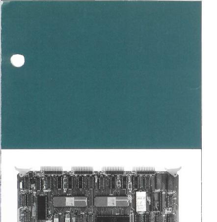
The MPC-4 is a S-100 bus intelligent multi-port communications board that provides four buttered RS-232C serial I/O channels to allow for multi-user and communications applications, and is controlled by the powerful Z80 microprocessor.
