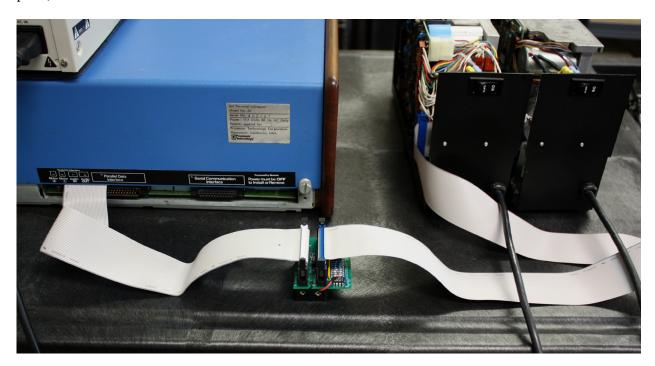
The VSG passes all signals between the controller and the drive except for index/sector pulses. Pulses from the drives are received by the VSG and the VSG generates the index/sector pulses that are seen by the controller. This arrangement is required to handle specific timing requirements expected by the controllers and software during the first revolution after a drive is selected.
