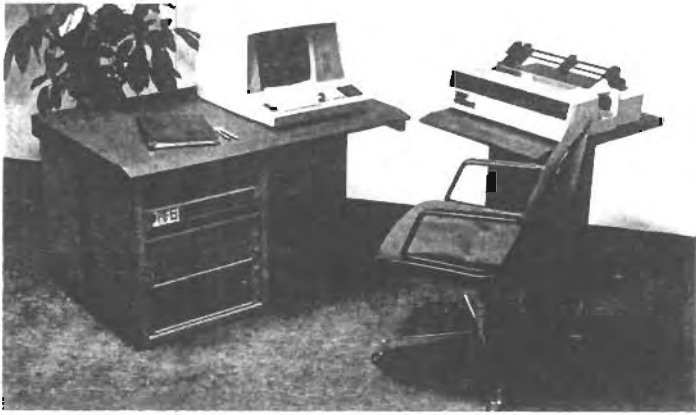
PERTEC COMPUTER CORPORATION's new MITS 300 Business System is comprised of a mainframe, a CRT terminal on a desk, and a line printer on a pedestal. Pictured here is the MITS 300/55, which is the hard disk, rather than the floppy disk, system.
