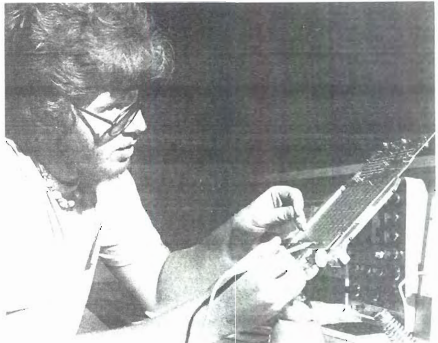
Kevin Stewart solders RAM IC sockets to 680-BSM circuit board.
