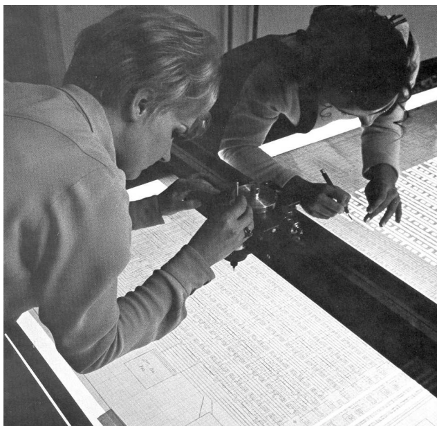
Figure 4: Technicians transferring layout to rubyolith
