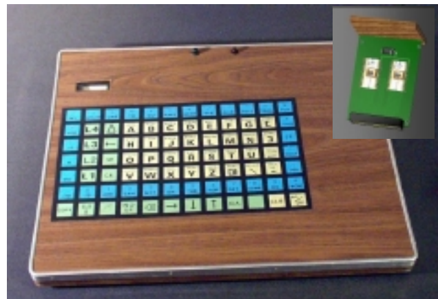
Figure 1: Autocomm and the word store using 1702A
