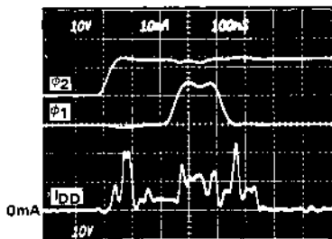
Figure 1. I_{DD} transient current during shift cycles. I_{DD} scale: 10mA/div.
