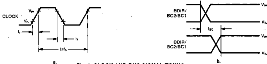
Fig. 9 CLOCK AND BUS SIGNAL TIMING
