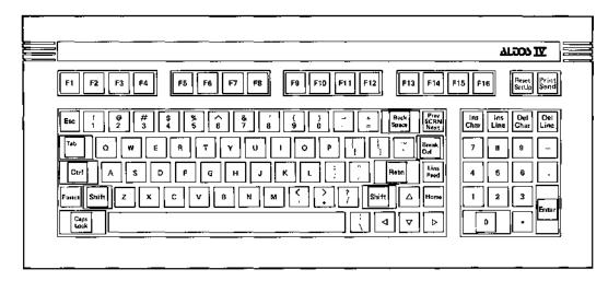
To reprogram the terminal control keys, see Chapter 2. The following table describes the default functions of the terminal control keys when the terminal's not in setup mode. The local keys, CAPS LOCK and RESET SETUP, act directly at the terminal. All the other keys (called remote keys) send ASCII codes that your computer's programs may reinterpret. If you are in block mode, the code is sent directly to the terminal and produces the effects described in Table 3.1.
