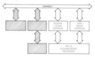
C. The third type are those devices designed for use with the positive-polarity input/output bus and the data-break facility of earlier PDP-8's. Because of special design features and reliable performance, these devices remain in demand for the new PDP-8's. As a result, DIGITAL has developed the I/O bus and data-break interfaces that allow the use of these desirable peripherals with the newest PDP-8's.
