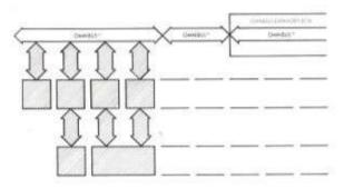
D. A full-blown PDP-8 system consists of many of each type of expansion device fied to the original OMNIBUS and its extensions. The basic -8/F and -8/M enclosures are smaller than that of the -8/E, and can accommodate only one OMNIBUS. Like the -8/E, however, an expander box can be added to bring the -8/F and -8/M capacity to 56 module slots.
