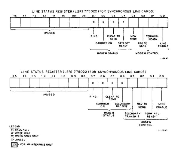
Figure 3-3 DV11 Primary Registers (Sheet 3 of 3)
