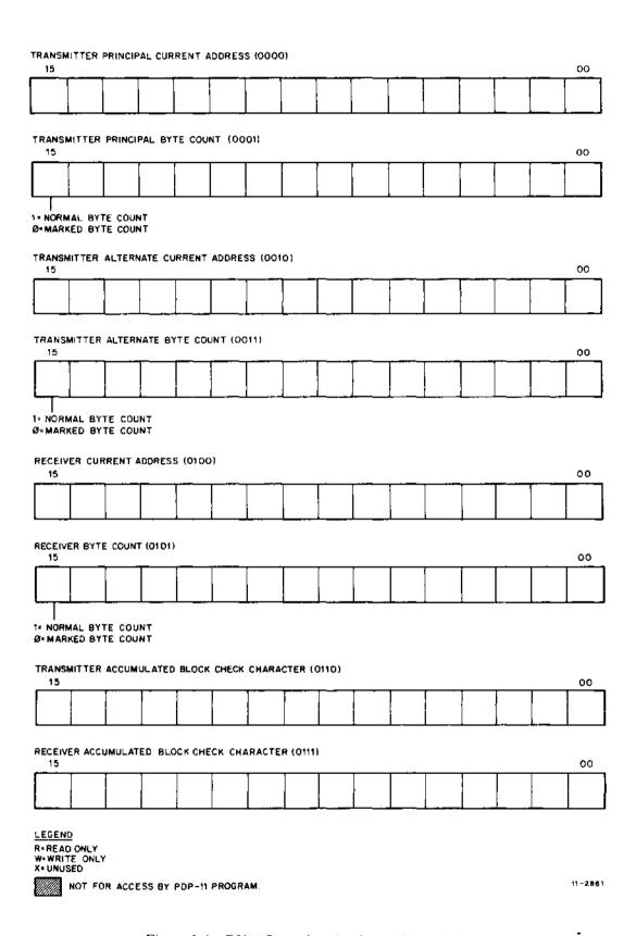
Figure 3-4 DV11 Secondary Registers (Sheet 1 of 2)
