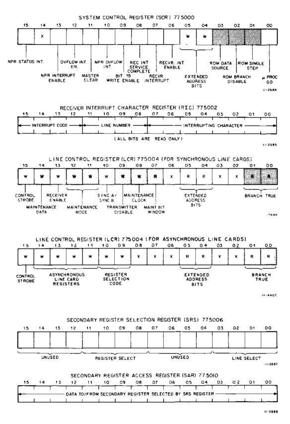
Figure 3-3 DV11 Primary Registers (Sheet 1 of 3)
