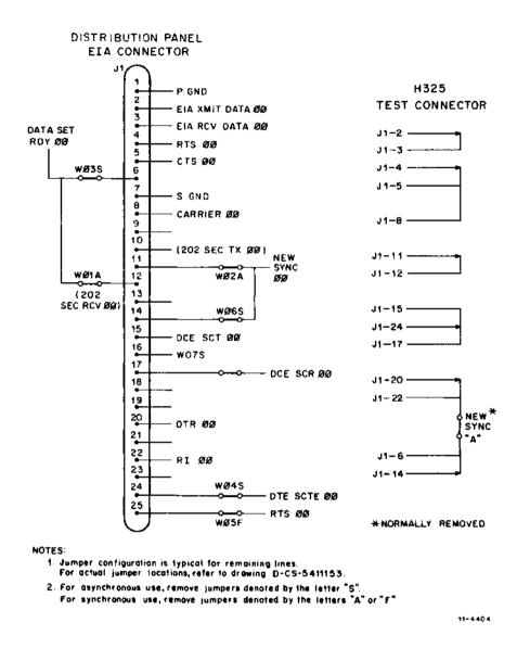
Figure 2-7 Distribution Panel and Test Connector Jumper Configuration
