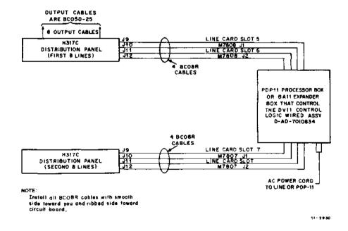
Figure 2-1 DV11 Interconnection Diagram
