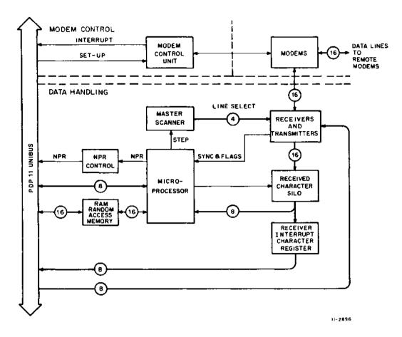
Figure 1-1 DV11 Overview Block Diagram
