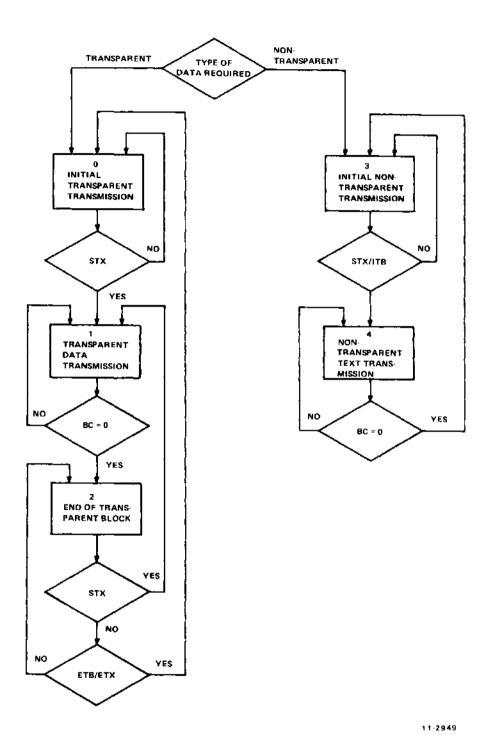
Figure 3-5 BISYNC Transmission Flow Diagram
