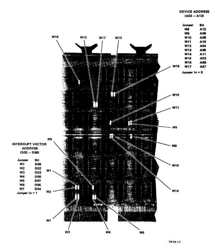
Figure 2-5 DV11 M7807 Module — Device Address Selection Jumpers and Interrupt Vector Address Selection Jumpers for DV11 Modem Control Unit
