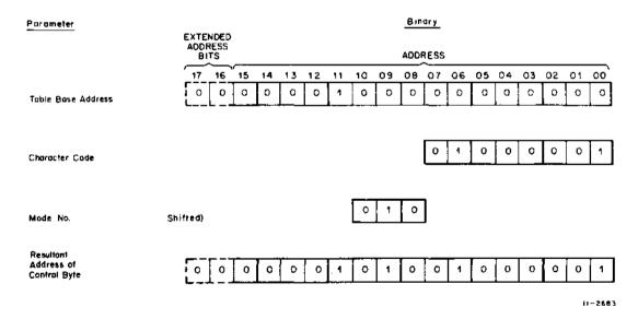
Figure 3-1 Control Byte Address
