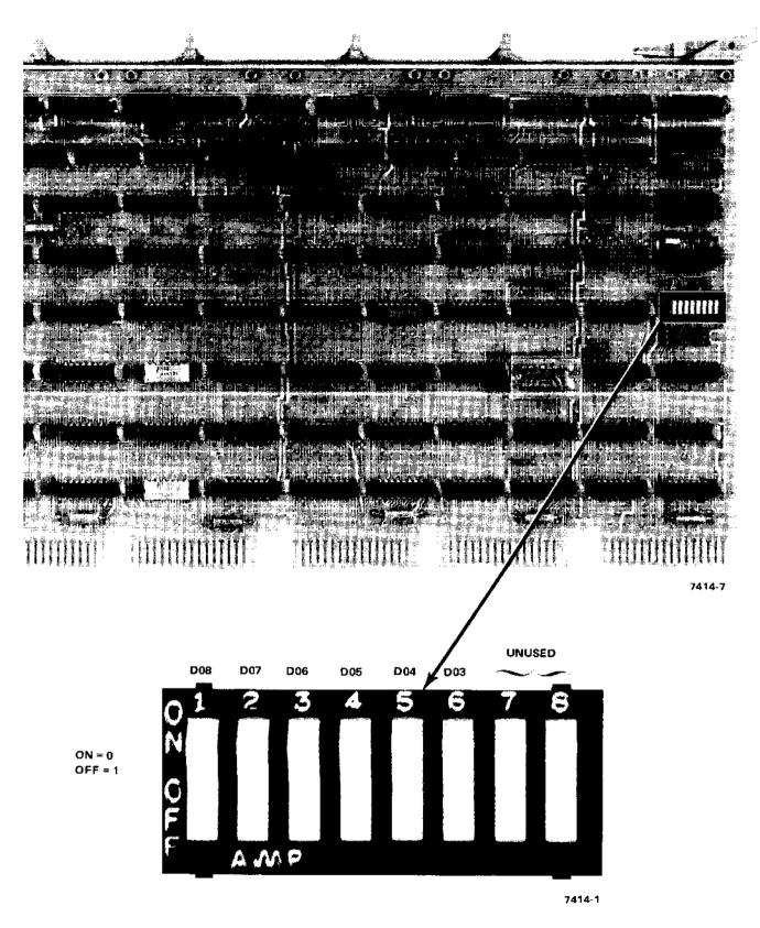
Figure 2-4 DV11 M7837 Module – Interrupt Vector Address Selection Switches for DV11 Data Handling Section
