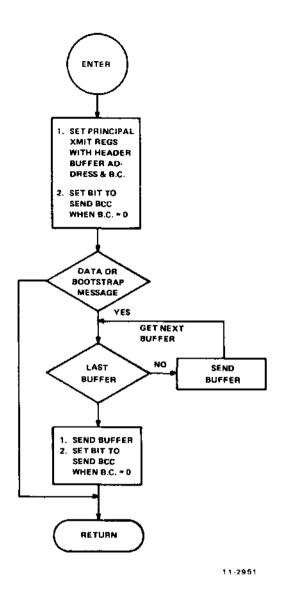
Figure 3-7 DDCMP Transmission Flow Diagram
