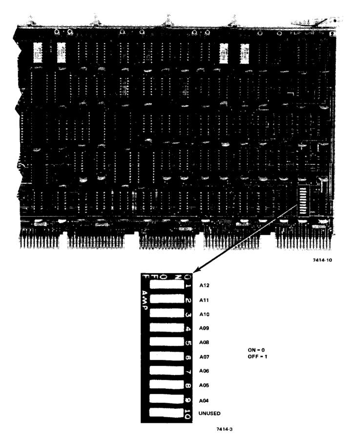
Figure 2-3 DV11 M7836 Module - Device Address Selection Switches
