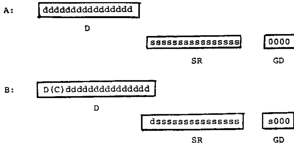
Figure 2-30: Right Shift on 32 Bits of Data
