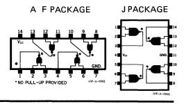
The 8881 is a Quad 2-Input NAND Gate with bare output collectors. Absence of an output pull-up structure allows the user complete freedom in the use of the 8881 in collector-logic (wired-AND) and similar applications. Proper pull-up resistor selection will allow as many as 50 outputs to be tied together.
