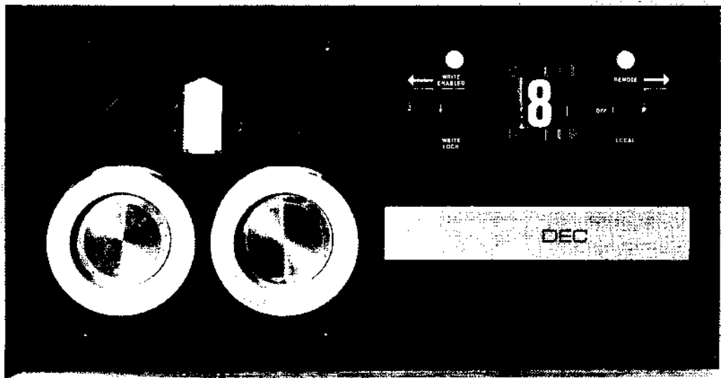
Figure INTRO-5 DECTape Transport Unit
