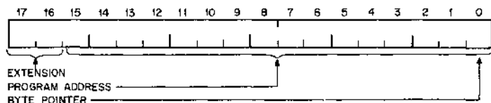
Figure 1-3 Address Line Bit Format
