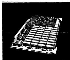
Uses 64Kb dynamic memory chips with large cell geometry for lowest soft error rate in the industry.
