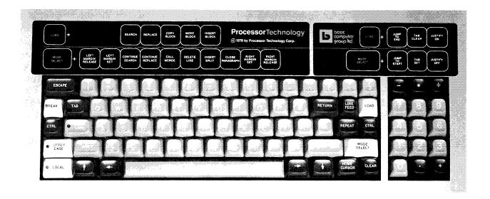
Stick the labels on the metal surface just above the Sol keyboard. Align the long label over the typewriter keyboard and the short one over the 15-key pad. For the long label, LOAD and MODE should be over the ESCAPE key, and RIGHT MARGIN RELEASE over the 0 key. For the short label, JUSTIFY OFF and JUSTIFY ON should be over the ÷ key of the 15-key pad.
