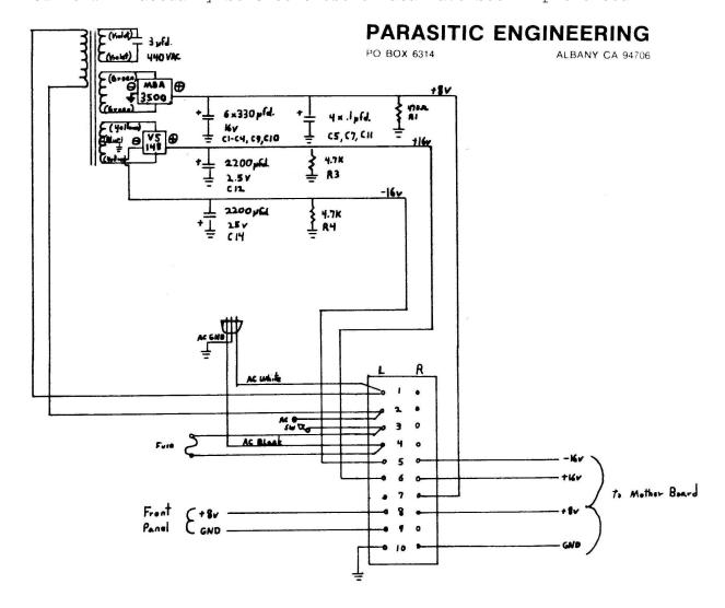
The trouble is that R4 is not actually wired as shown. If the Parasitic Engineering instructions are followed, the circuit is actually like this (Note the incorrect position of R4):
