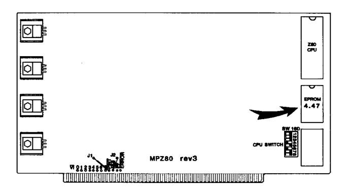
To insert the new PROM, with the notch oriented toward the top of the board, line up the pins on one side of the PROM with the row of pin sockets and insert the pins partway. Then, lineup the other row of pins with their sockets and insert them partway. The rows of pins usually tend to be bent away from each other slightly, so inserting the second row of pins will require you to push the chip against the first row of pins until the second row can be inserted in the socket.
