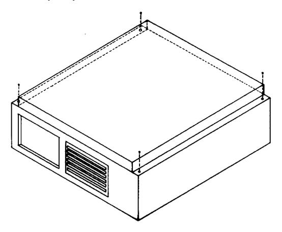
Remove the four screws completely and put them in a safe place away from the cabinet. Then, turn the cabinet right side up and slide the cover forward. When the cover is almost completely off, you will need to move it from side to side to get it off completely.
