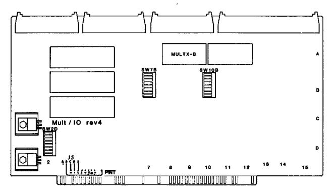
With this wire in place, your MULT I/O can transmit interrupt requests to the MPZ-80 board. When the MPZ-80 acknowledges the interrupt, the MULT I/O provides the address of the service routine. This is enabled by having a slide jumper connecting the pins B and C at J4. If your board has these jumpers, you are ready for Micronix.
