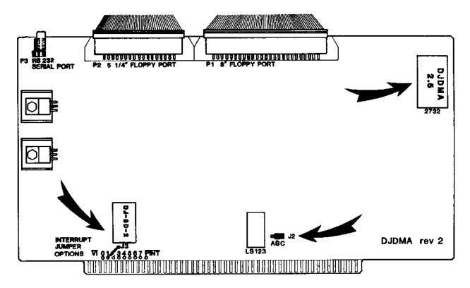
There should be a wire connecting the point labeled J3 with the point labeled 1. If there isn't a wire there, you will need to solder an insulated wire between these two points. This wire connects the interrupt signal from the DJ/DMA to vectored interrupt 1.
