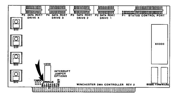
There should be a wire connecting the point labeled J5 and the point labeled 0. This wire connects interrupt requests from the HDC/DMA controller to vectored interrupt line 0. If this wire isn't here, you will need to install it. The wire must be soldered in place, and be insulated except at the ends. If you aren't an expert solderer, have a skilled friend (or technician) do it for you.
