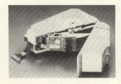
bearings on both top and bottom of the spindle and the positioner allow track density of 1207 tpi and recording density of 19077 bpi. With capacity up to 300 Mbytes per drive and a 25 msec average positioning time, the MegaFile has a 25000 hours HDA Mean Time Between Failure (MTBF). **Siemens**, West Lake Village, CA
