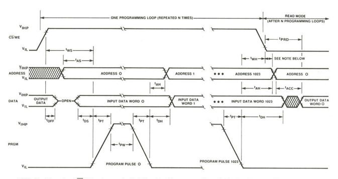
NOTE: The falling edge of  $\overline{\text{CS}}/\text{WE}$  must occur after the falling edge of the program pulse and before the address transition.
