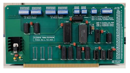
From 0000-7FFF, RAM can start on any 1K boundary and extend from that address through 7FFF. This allows keeping small RAM boards in your system (e.g, 1K, 4K) and having the FLEX64K board fill above those boards with RAM.
